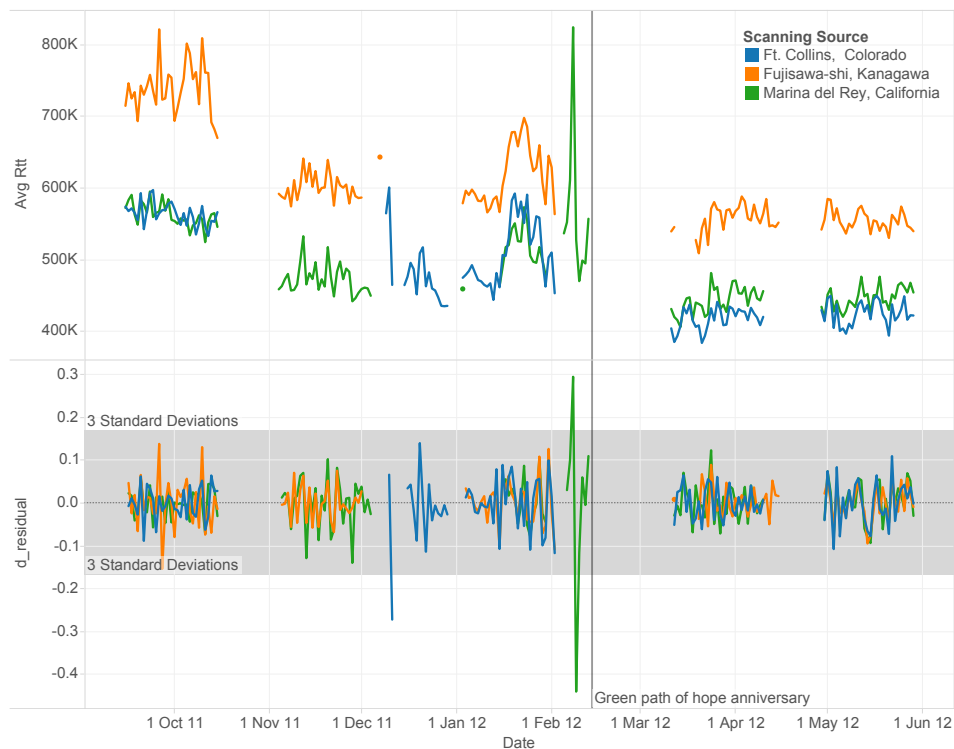
Figure 2: Census: Average ping times and world traffic corrected difference residuals in Tehran and a mobile phone ISP pre and post the anniversary of the green movement. Based on 596,733 census probes.
