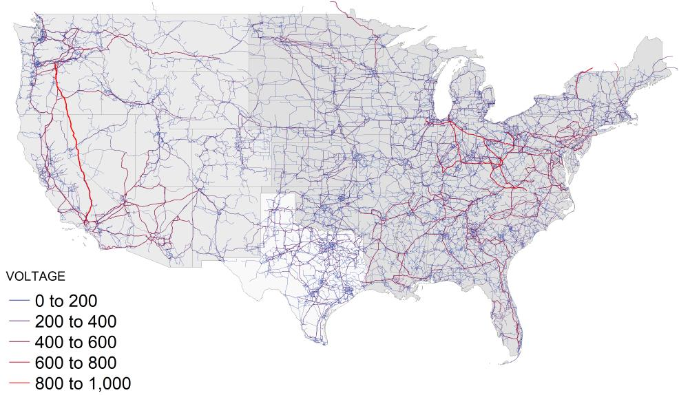
Notes: This Figure shows the high voltage transmission network of the United States as well as the interconnections between the networks using data from the U.S. Energy Information Administration. While there are a few small interconnections between the three networks, they are effectively independent.
