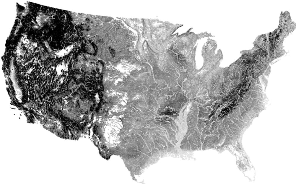
Notes: This figure plots the sources of waterpower potential in the United States, with darker shares corresponding to greater flow rates or fall heights. Panel A plots our estimated flow rates for each river segment, in cubic feet per second. Panel B plots the drop in elevation for each river segment, in feet per mile. Data from NHDPlusV2.
