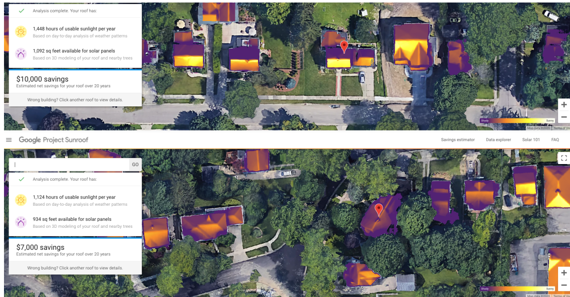
Figure 4: Google Project Sunroof display. (Top) shows example readout for the home marked with location flag. This home enjoys unobstructed sunlight and has a large, flat, south-facing roof segment. Google Sunroof predicts substantial savings when installing solar on this home. (Bottom) this home has extensive shading and does not have a substantial south-facing roof segment. Google Sunroof predicts lower savings when installing solar on this home. These homes are in the same neighborhood in East Lansing, Michigan, and are served by the same electric utility.
