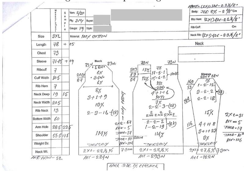
**Note:** The figure shows a sample design chart of a sweater that the workers use to knit sweaters, and which we used to estimate SMVs for the corresponding sweaters.
