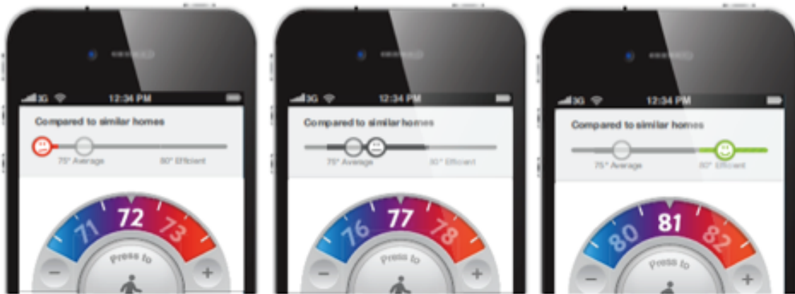
(a) Setpoint Choice Messaging: Screenshots of smartphone app that shows the messaging associated with different temperature set points.
