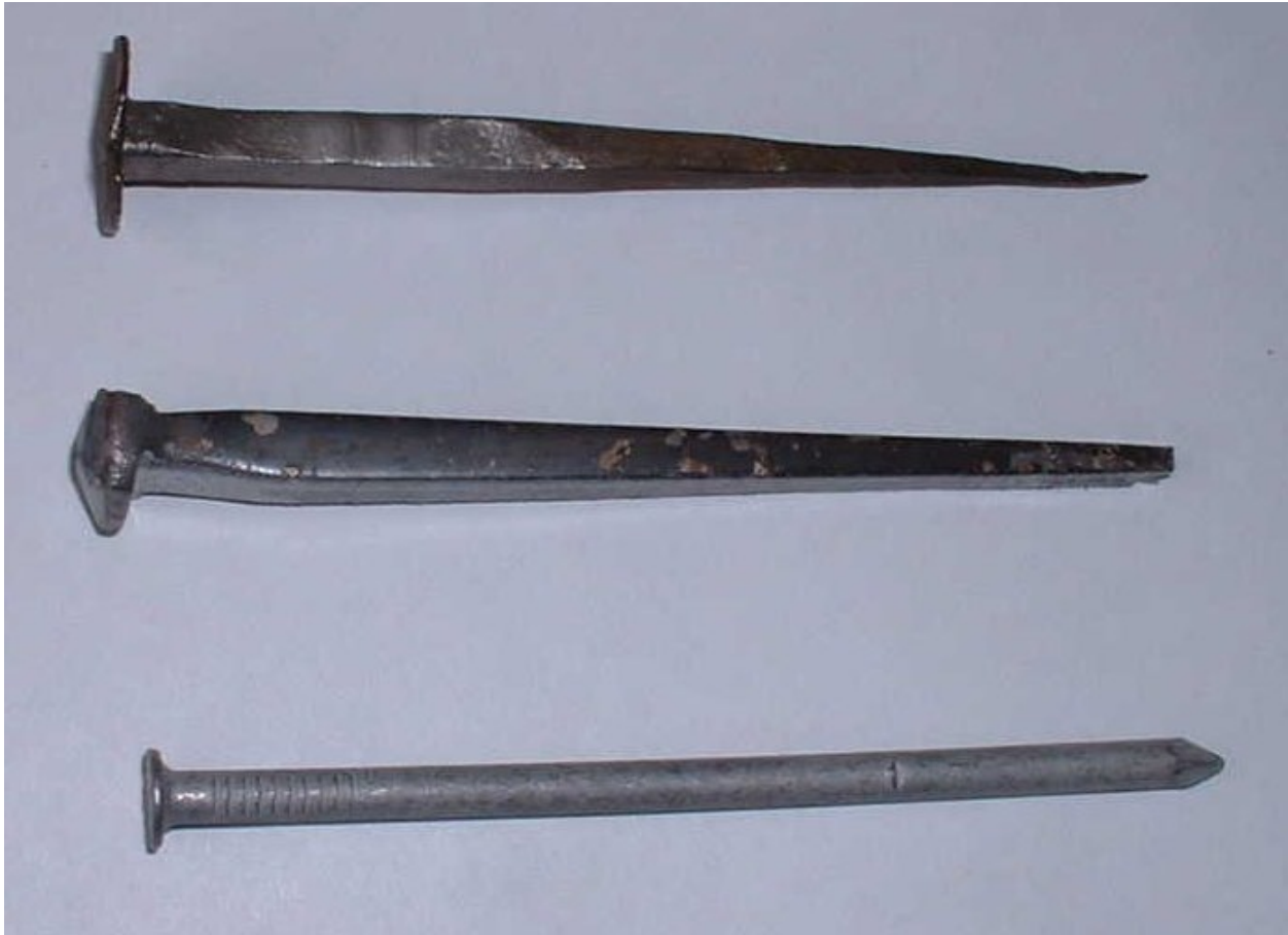
Figure 2 Hand Forged, Machine Cut, and Wire Nails
