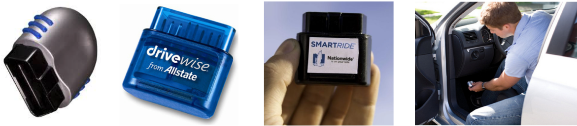
Figure A.1: Examples of Telematics Devices in U.S. Auto Insurance
