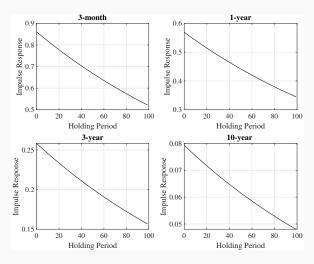
Response to 1 bps. shock to short rate. Holding period in months. Response for  $\phi{=}0.9{:}\ \frac{\Delta y_{t+k}^{N,RE}}{\Delta r_s^{\xi}} = \frac{1}{N} \frac{1-\phi^N}{1-\phi} \phi^k.$
